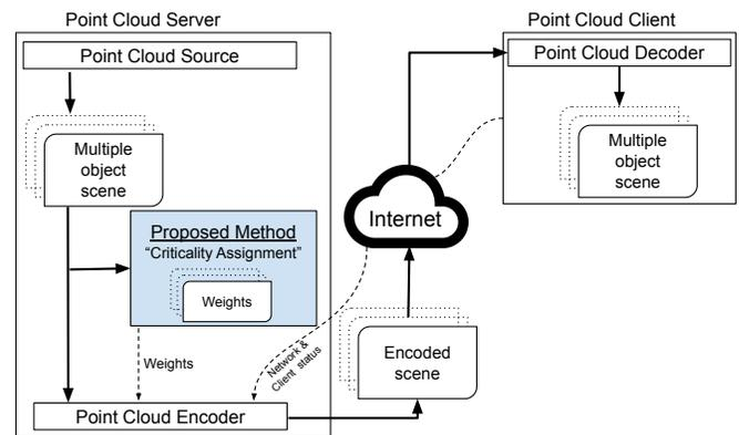
Fig. 3. High-level architecture of point cloud streaming system incorporating our proposed method.
