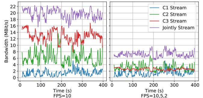
Fig. 8. Bitrates savings by adopting frame rates 10, 5, and 2 for criticality 1, 2, and 3 points, respectively, against fixed frame rate for all points.
