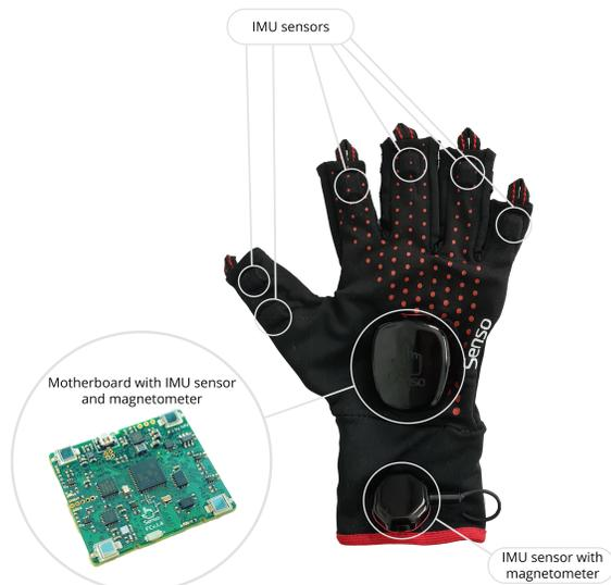
Fig. 2. Data glove used in this work: *Senso Glove DK2*
