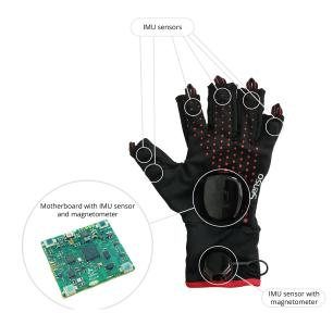
Fig. 2. Data glove used in this work: Senso Glove DK2
