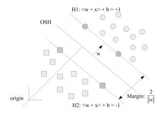
Fig. 3. OSH: Optimal separating hyperplane. By maximizing the margin between data of both classes, the error rate of classifying unseen data can be minimized [8].
