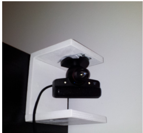
Fig. 6. Playstation Eye camera out-of-the-box (left) and hanging upside-down in the custom-built stand (right)
