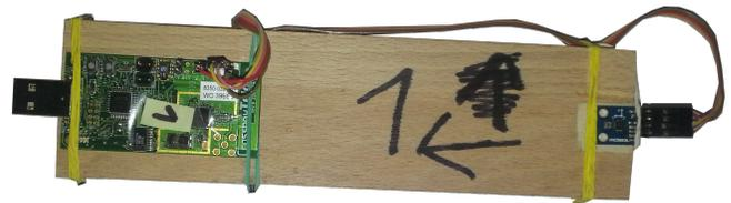
Figure 4: TelosB mote setup with the HMC5883L sensor mounted on a wooden block.
