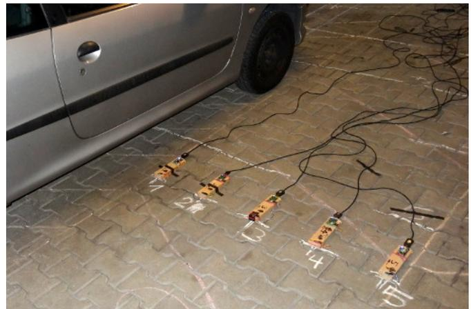
Figure 8: Measurement setup for distance measurements.
