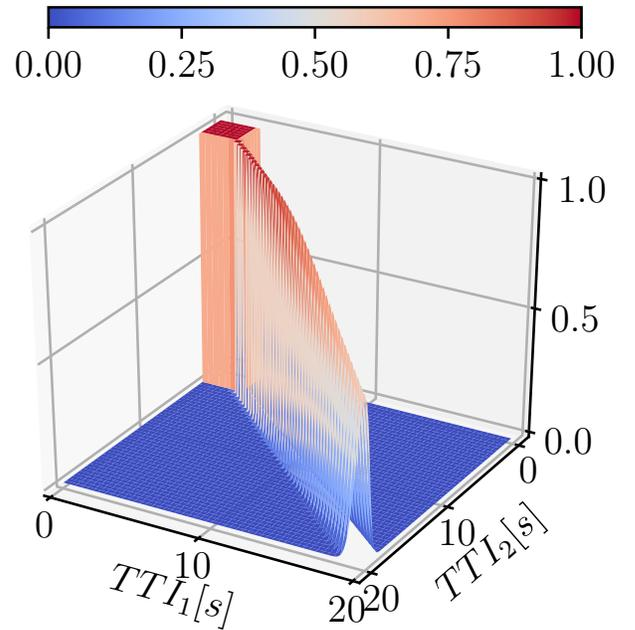
Fig. 3. Relevance function for two vehicles with their respective TTIs. The relevance is highest if the vehicle both vehicles are close to the intersection.
