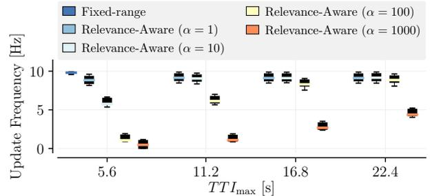
Fig. 5. *FCD Update Rate* depending on the scale factor  $\alpha$  and the maximum TTI  $TTI_{\max}$ . On the left, the baseline approach is displayed. The Update Rate of our approach depends on the parameters, but is always slightly lower compared to the baseline.
