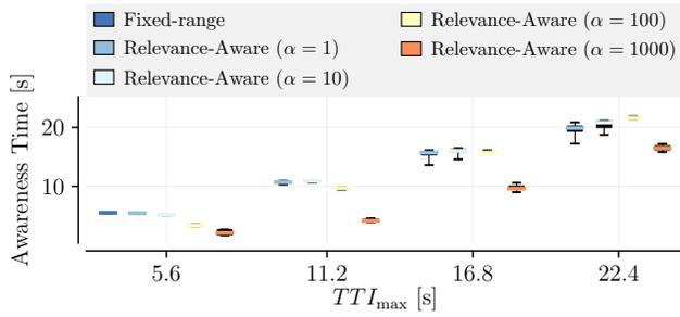
Fig. 6. Awareness Time depending on the scale factor  $\alpha$  and the maximum TTI  $TTI_{max}$ . On the left, the baseline approach is displayed. Our approach provide information about potential collisions much early, which can improve the decision-making of the vehicles.
