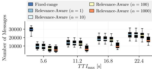
Fig. 4. *Number of Messages* depending on the scale factor  $\alpha$  and the maximum TTI  $TTI_{\max}$ . On the left, the baseline approach is displayed. Our approach uses significantly less bandwidth.
