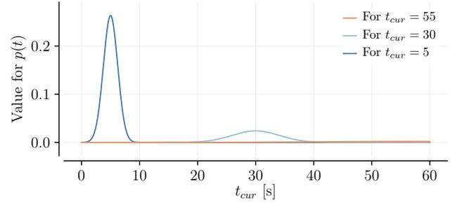
Fig. 2. Distribution of TTI for  $\alpha = 1000$  and  $TTI_{max} = 60$ . The  $\sigma(t_{cur})$  decreases with decreasing  $t_{cur}$
