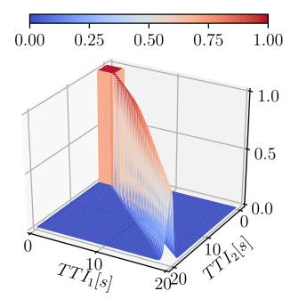
Fig. 3. Relevance function for two vehicles with their respective TTIs. The relevance is highest if the vehicle both vehicles are close to the intersection.
