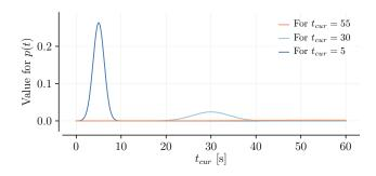
Fig. 2. Distribution of TTI for  $\alpha = 1000$  and  $TTI_{\rm max} = 60$ . The  $\sigma(t_{\rm cur})$  decreases with decreasing  $t_{\rm cur}$
