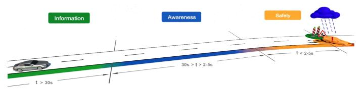
Figure 1: Visualization of our three derived zones of information demand for communication based ADAS. The classification is related to the maximum allowed latency from the earliest detection of information till the usage in the assistance feature.
