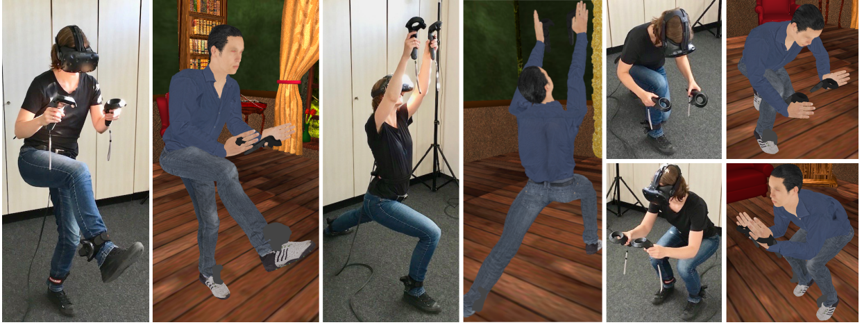
Fig. 5: Examples of our real-time full-body motion reconstruction based on HTC Vive trackers and controllers.
