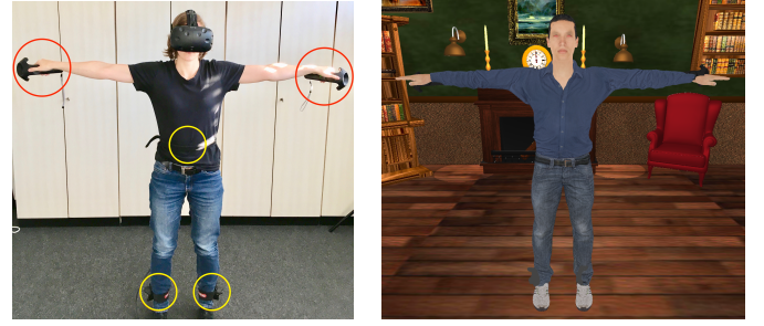
Fig. 1: Calibration process: A student is standing in a T-pose and holding two Vive controllers (red), while three trackers are bound to the feet and hip (yellow).
