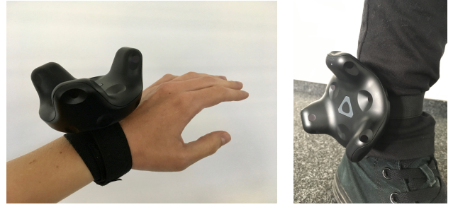
Fig. 5 Strapped Vive Tracker during the evaluation (left). To track the leg movements, an additional Tracker must be strapped to the ankle.
