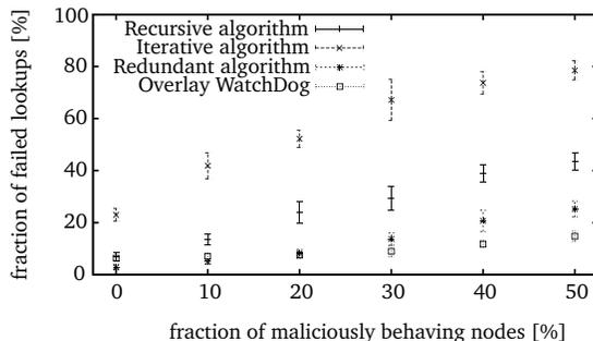
**Fig. 6.** A comparison between the different security mechanisms
