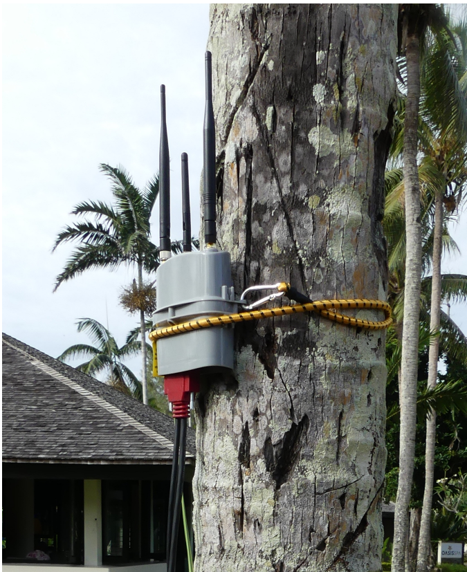
Fig. 6. A third-generation of the Serval Mesh Extender, in its natural environment, strapped to a coconut palm in Vanuatu.
