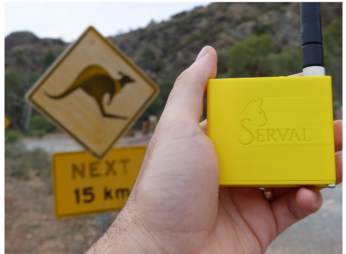
Fig. 2. A second generation Serval Mesh Extender prototype, looking more communicative and less explosive than the first. The 3D-printed exterior gives the appearance of a more advanced prototype. Internally, however, it still consists entirely of carefully selected off-the-shelf components.
