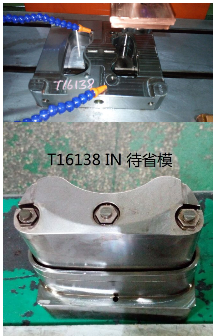
Fig. 4. Injection-molding tools during the milling process (top), and on completion. The complete set of tools consisted of several such pieces.
