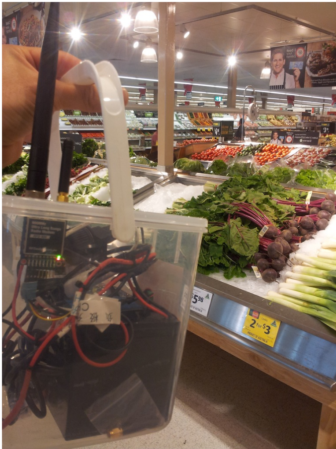
Fig. 1. The original Serval Mesh Extender prototype, during an indoor test at the local supermarket, where the plastic tub was purchased. This prototype was built entirely from off-the-shelf products.
