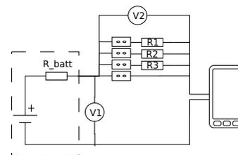
Figure 1. Schematic of the measurement circuit.
