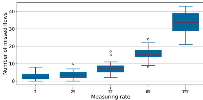
Fig. 7: The number of undetected/missed subflows with different measurement interval lengths (measurement rate).
