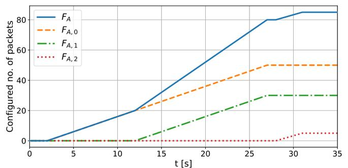
Fig. 3: Accumulated packets dispatched from the sender over time: Flow  $F_A$  consists of three subflows  $F_{A,0}$ ,  $F_{A,1}$ , and  $F_{A,2}$ .
