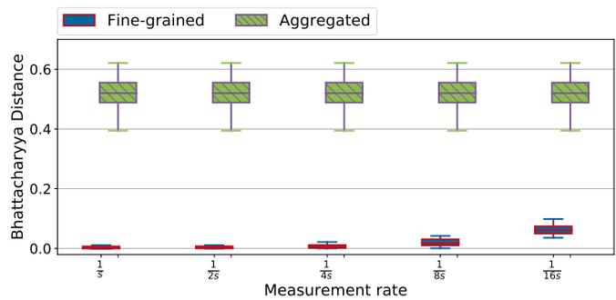
Fig. 6: Accuracy in terms of Bhattacharyya distance between ground truth and measurements for the FSD applying the proposed fine-grained measurement approach and aggregated measurements with different measurement rates.
