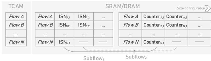
Fig. 1: Registers set up tables to (i) store the ISNs of SYN packets to identify subflows and (ii) to count packets for the corresponding subflows.
