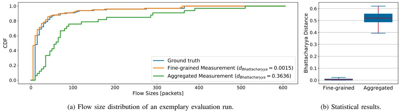
Fig. 5: Accuracy comparison using the measured flow size distribution of the proposed fine-grained measurement approach with aggregated measurements. The actually dispatched application-level flows are used as ground truth.
