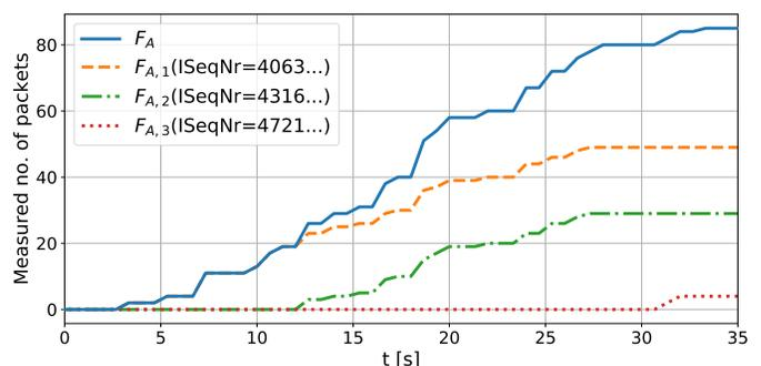
Fig. 4: Accumulated packets visible in the switch over time compared to Figure 3. The switch correctly detects three flows and distinguishes their traffic.
