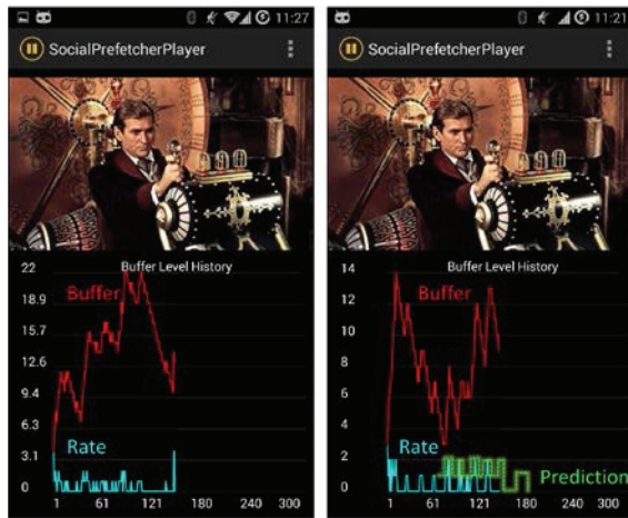
Figure 4: Left side: Normal player internal. Right side: Prediction-based optimized player.
