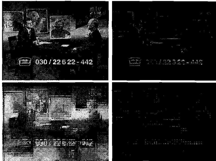
Figure 5: Video clip "talk" original (top left), 1 DCT coefficient protected (right), 1 VLC bit encrypted (bottom left), combination of both (right)
