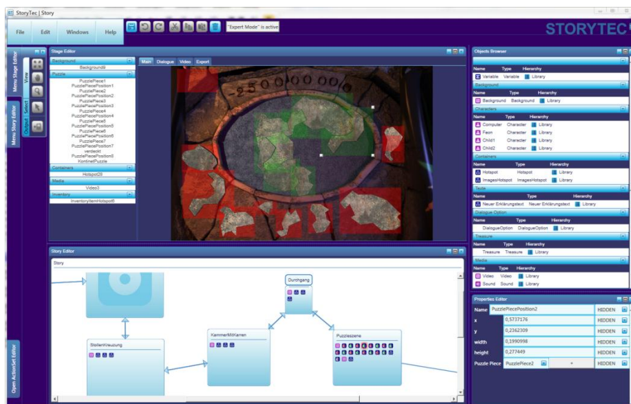
Fig. 2. StoryTec used for authoring a puzzle in an educational adventure game. The editors shown in this figure and figure 4: Stage Editor (upper left), Story Editor (lower left), Objects Browser (upper right) and Property Editor (lower right)
