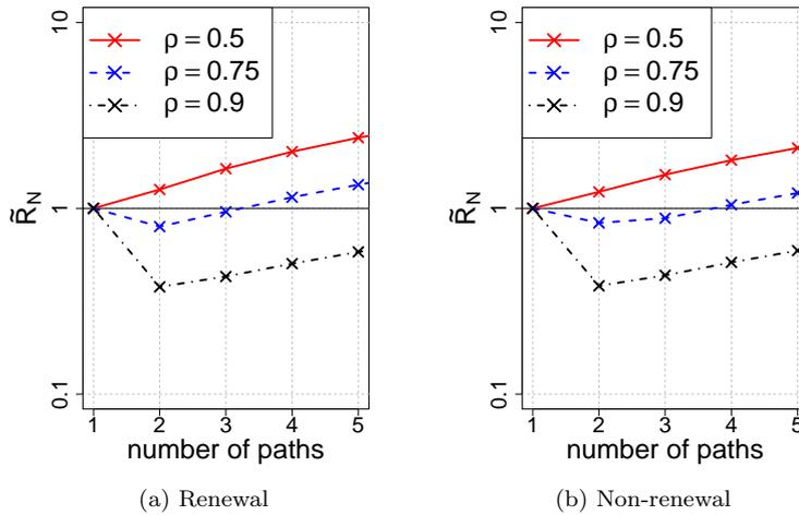
**Fig. 10** Multipath routing reduces the average batch response time when  $\tilde{R}_N < 1$ ; smaller  $\tilde{R}_N$  corresponds to larger reductions. Baseline parameter  $\mu = 1$  and non-renewal parameters:  $p = 0.1, q = 0.4, \lambda_1 = \{0.39, 0.7, 0.88\}, \lambda_2 = 0.95$ , yielding the utilizations  $\rho = \{0.5, 0.75, 0.9\}$  (from top to bottom).
