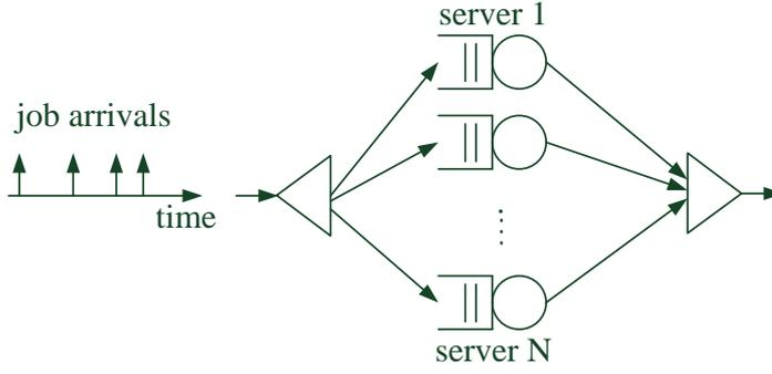
**Fig. 2** A schematic Fork-Join queueing system with  $N$  parallel servers. An arriving job is split into  $N$  tasks, one for each server. A job leaves the FJ system when all of its tasks are served. An arriving job is considered waiting until the service of the last of its tasks starts, i.e., when the previous job departs the system.
