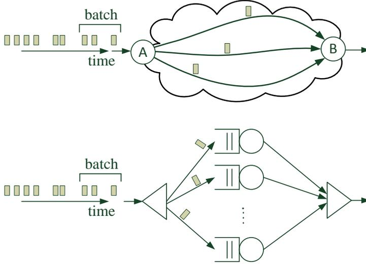
**Fig. 9** A schematic description of the window-based transmission over multipath routing; each path is modelled as a single server/queue.
