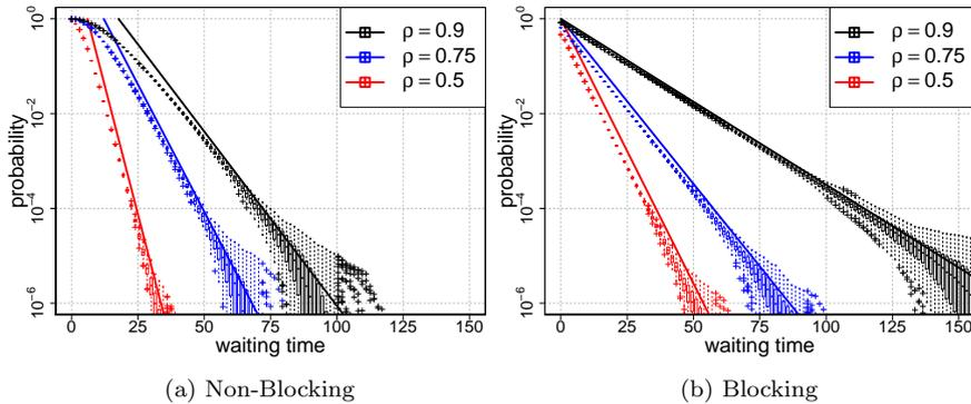
**Fig. 6** Bounds on the waiting time distributions vs. simulations (non-renewal input): (a) the non-blocking case (25) and (b) the blocking case (31). The parameters are  $N = 20$ ,  $\mu = 1$ ,  $p = 0.1$ ,  $q = 0.4$ ,  $\lambda_1 \in \{0.4, 0.72, 0.72\}$  and  $\lambda_2 \in \{0.9, 0.9, 1.62\}$  leading to utilizations  $\rho \in \{0.5, 0.75, 0.9\}$ . Simulations include 100 runs, each accounting for  $10^7$  slots.
