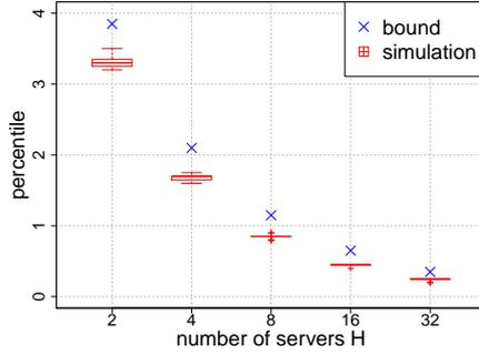
**Fig. 7** Round-robin partial mapping: Bound on the waiting time percentile  $w^\varepsilon$  for renewal arrivals and increasing number of servers (fan-out)  $H$ . The system parameters are  $\mu = 1$ ,  $\lambda = 0.75$ ,  $\varepsilon = 10^{-3}$  and the overall number of servers is  $N = 2^8$ .
