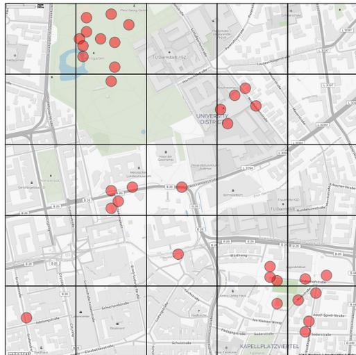
Fig. 2: Grid overlay with location measurements in an inner-city environment. The grid size and its placement have a significant influence to which cells measurements are allocated to. Some groups are within a single cell, while others are spread over multiple cells.
