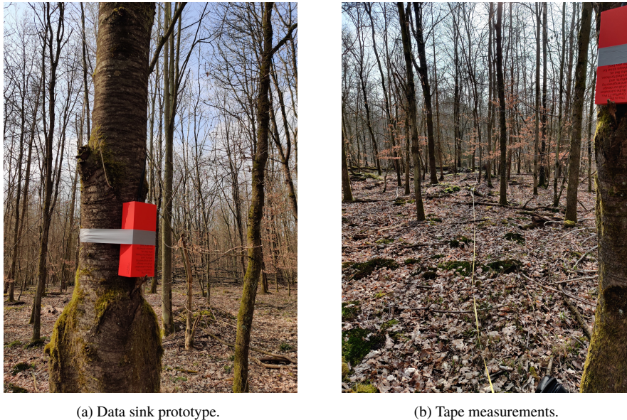
Fig. 2: The data sink prototype was attached to a tree at around 1.80 m height. Distances were measured with a tape measure in a German mixed forest.
