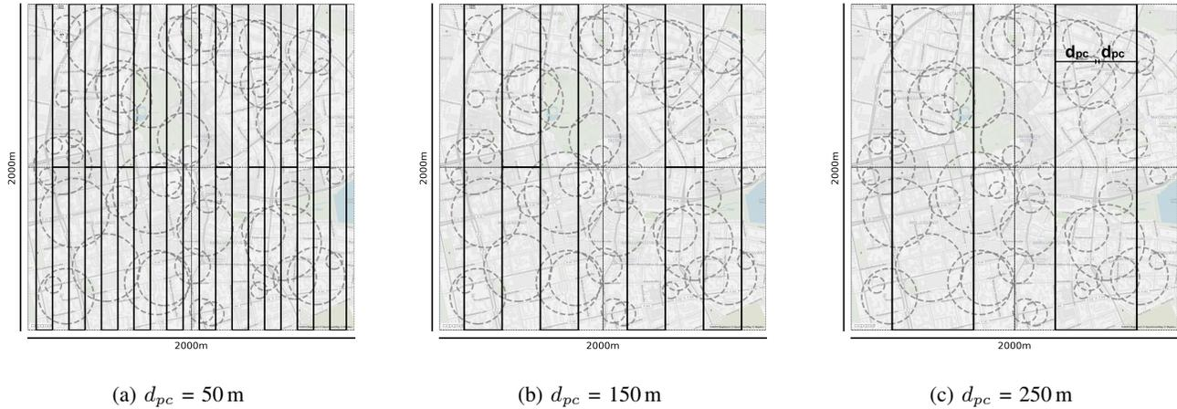
Fig. 2: The operation area is divided into four square-shaped monitoring areas. The lawnmower pattern is used to calculate flight paths of monitoring UAVs, shown in black. The strips of the flight paths are separated by a path clearance distance  $d_{pc}$  on each side. The distribution and extent of points of interest of the used mobility model for all simulation runs is shown in the background as grey circles.
